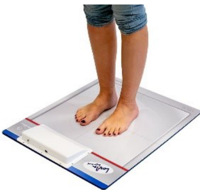
Figure 5. EPS R2 pedobarograph used in the study. Source: PODOLOGIA.PL
