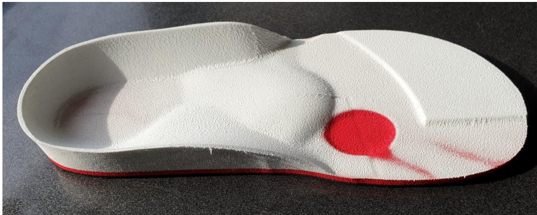
Figure 10. Final view of a) insole designed in RhinoCeros (Insoles 3D) – LutraCad, b) manufactured insole
